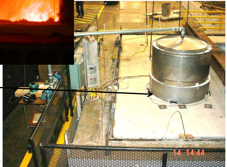
View into furnace during engulfment test
