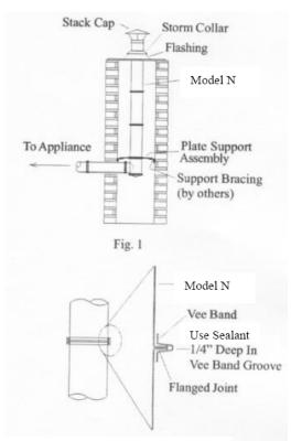
Assembled Model N Joint Detail
